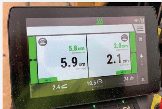
LA MODALITÀ A SCHERMO DIVISO DEI DISPLAY DEL CAT GRADE CONTROL PERMETTE DI MONITORARE FACILMENTE ENTRAMBI I LATI DEL BANCO.
